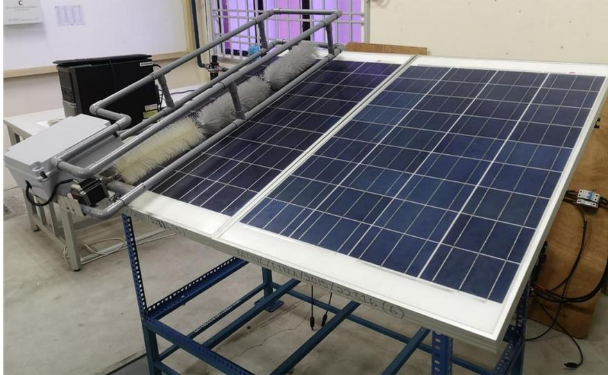
Figure 1. Solar panel cleaning machine
