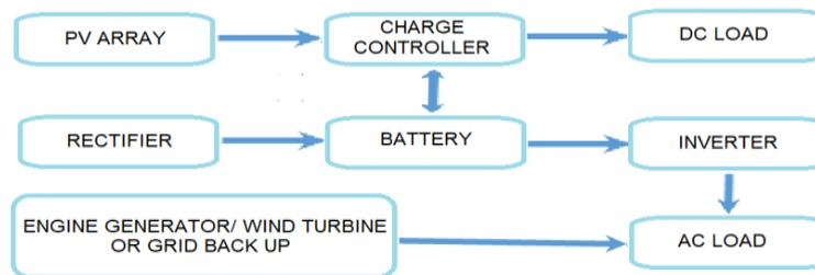
Figure 4. Diagram of PV hybrid system
