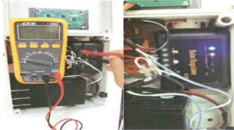
Figure 21. Power input to the solar charger controller
