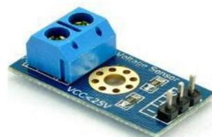
Figure 9. Voltage Sensor
