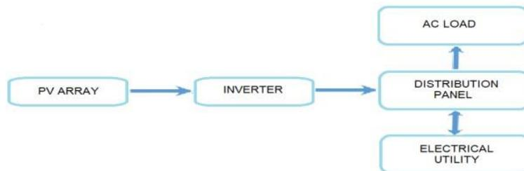
Figure 1. Block Diagram of grid-connected PV System
