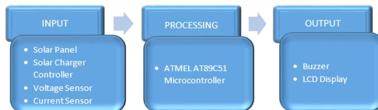
Figure 6. Block diagram of stand-alone PV system
