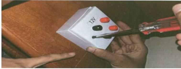
Figure 19. Installation of banana socket at every workstation
