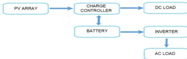
Figure 3. Diagram of stand-alone PV system with battery storage powering DC and AC loads
