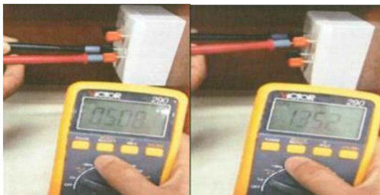
Figure 22. Voltage value of each pair of banana socket at the workstation
